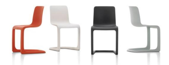
EVO-C is a successful, uncompromising iteration of the principle and characteristics of the classic cantilever chair in the material of plastic. Thanks to today's gas injection moulding technology, plastic structures can achieve the proven strength and rigidity of cantilevered tubular steel constructions. The load-bearing structure is formed by hollow tube-like components that flow seamlessly into the planar surfaces of the seat and back.
