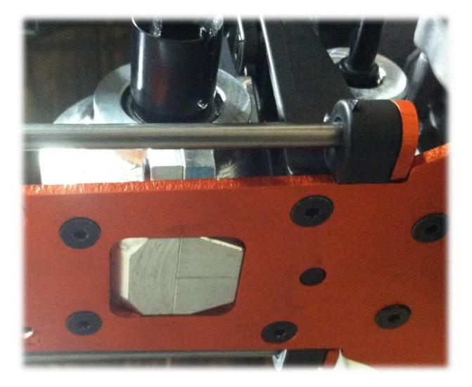
11. Assemble remainder as you would stock transmission per HPI instructions. After you assemble the transmission top plate, install and tighten 1pc-M4x12 Button head with M4 flat washer. Finish assembly.
