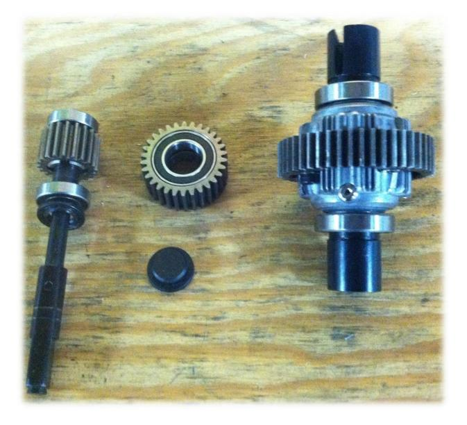
3. HPI gear shaft seal #86667 is optional, I recommend using it for added protection. Also, now is the best time to replace any worn parts.
