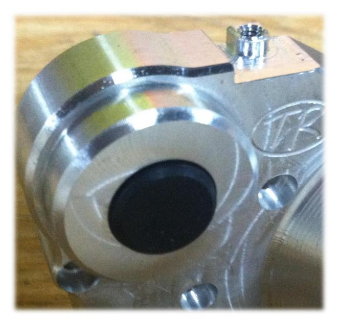
6.Assemble left half of TR transmission onto right half assembly. This may take some wiggling and finesse to make everything fit together. The transmission halves should mate easily; there may be a slight gap when they touch. Install the 4pcs.-M4x15 Socket heads; screw each one a little more to draw transmission halves together. Do not tighten one all the way, tighten each screw evenly. Once transmission halves are completely seated, tighten all 4 socket heads.
