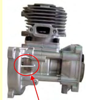
Added a rib on the muffler side of crankcase
