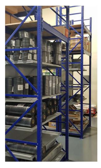
Longspan racking is ideal when products are handled manually rather than by forklift truck. The beam loading capacity is generally less than pallet racking although most weight loadings are available. Palletised products can be stored at floor level with the loose stock being stored above.
