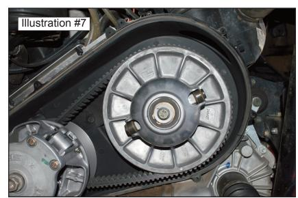
D-4. Install the belt. (SLP recommends **Polaris Belt #3211148 on 2014 models or Polaris Belt #3211180 on 2015 models** for proper operation)
