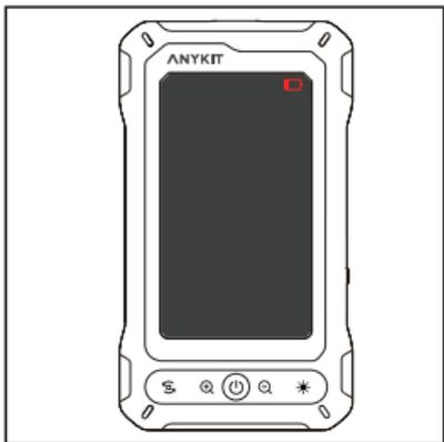
**Step 3:** Low Battery Indicator (If the battery icon on the screen shows low battery, please charge it fully before using it).
