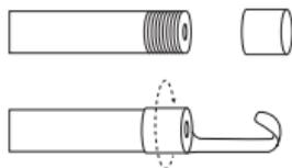
Unscrew the thread protector, then screw on the accessory.
