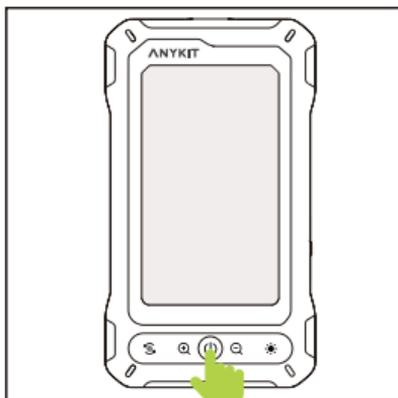
**Step 2:** Switch the Camera On/Off (press and hold the “
