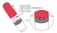
Turn the battery cover clockwise to align the arrow symbol with the unlock mark. Then take off the battery cover to install 6 AAA batteries into the battery compartment.
