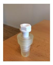
Valve screw is open and cannot get further out of the valve.
