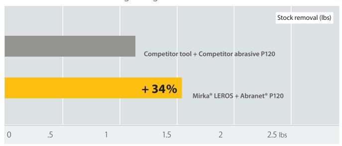
Comparison of stock removal between Mirka LEROS (Abranet P120) and a comparable competitor tool (abrasive grit P120).
