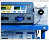
E3600 sensor synchronizes the OptiMumm™ smoke evacuator with any electrosurgical generator
