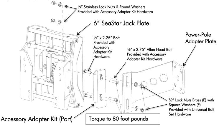
**Step 3** Mount the Power-Pole shallow water anchor to the adapter plate by following the mounting instructions in the hardware kit for adapter plates.
