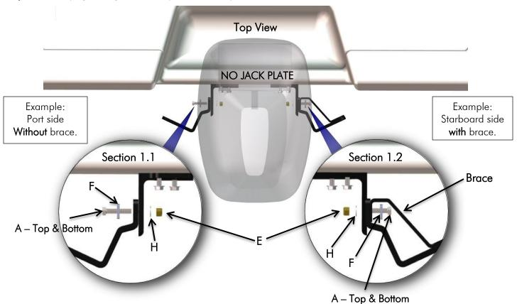
**Step 4** Mount the Power-Pole shallow water anchor to the adapter plate by following the mounting instructions in the hardware kit for adapter plates.
