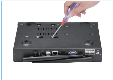
③ Screw HDD to the bottom
