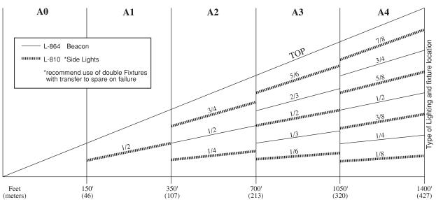
NOTE: Lowest level of lights must be raised above the height of adjacent structures. If your structure is not represented, allow us to assist you with selecting the proper products for your specific structure. Example: For structure "A1", one L-864 beacon is required at top and L-810 sidelights are to be mounted at ½ tower height.
