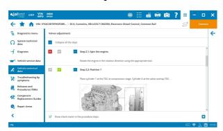
New engine type data, vehicle service data and technical procedures such as the distribution phasing, valve adjustment, fuel filter change, rocker arm disassembly and assembly or coolant filling/bleeding.
