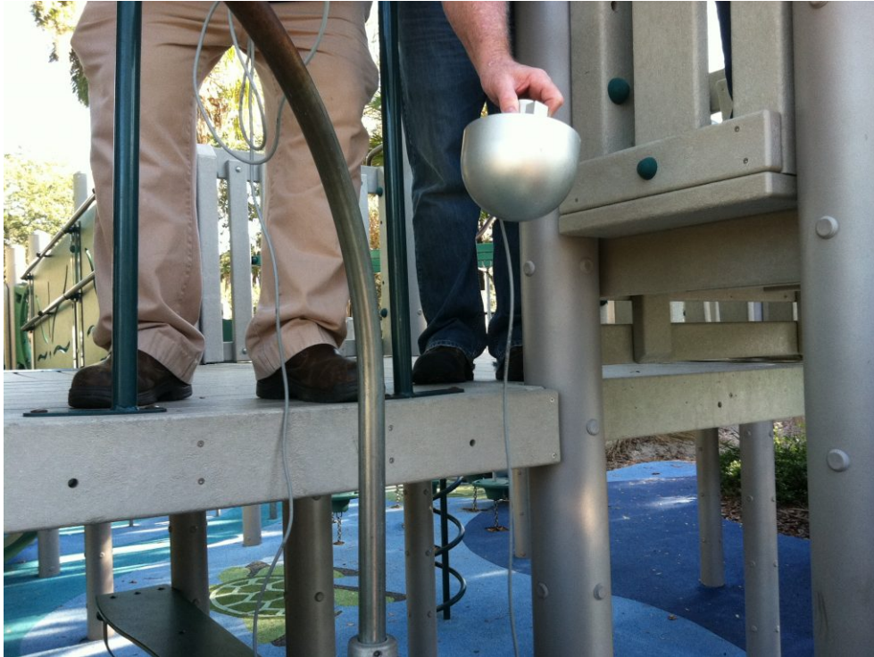
A ball form about to be dropped to measure HIC and GMAX
