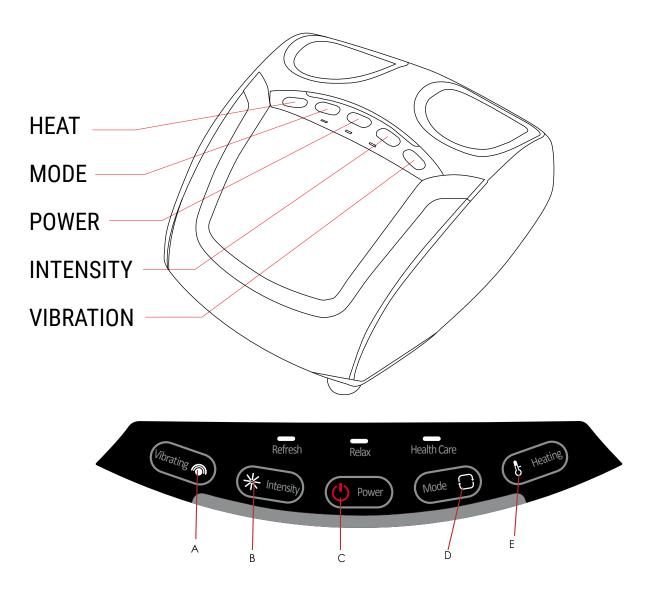
A) Vibrating Button: Controls Vibration Patterns
