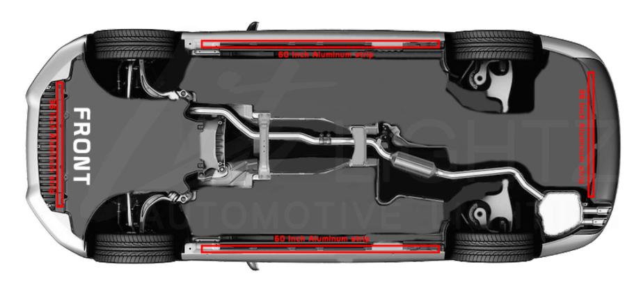
\*Note\* For the aluminum brackets to hold the aluminum strip, the brackets will need to be clip to the 2-second row on the side of the aluminum strip. You will hear it clip if you mounted them correctly. Depending on the vehicle, you may or may not have a flat surface on the rear of the car. If this is the case, please mount the LED strip using zip ties and the 3M tape on the back of the strip.
