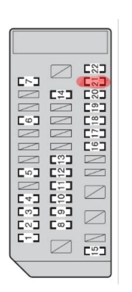
Note: By connecting the Fuse Tap to the location mark on the picture below, your Footwell Kit will turn on when the ignition is on and turn off when the ignition is off.
