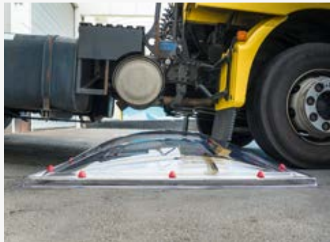
Test with Skylux polycarbonate armoured skylight: the skylight does not break, but returns to its original form instead
