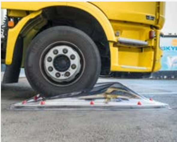
Test with Skylux polycarbonate armoured skylight: the skylight does not break, but returns to its original form instead
