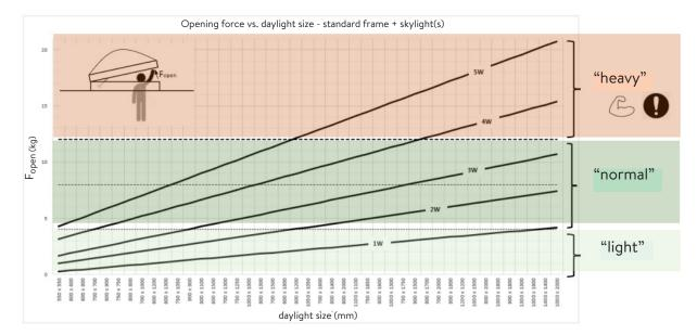
Graph: standard PVC frame in combination with 1-, 2-, 3-, 4- or 5-walled skylight:
