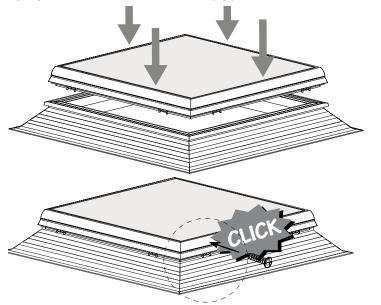
For extra reinforcement, screw the clips through the curb with delivered screws.
