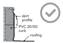
**OK:** roof covering is pulled up to below the skirt profile
