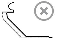
**Incorrect:** roof covering is pulled up over the flange
