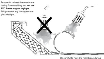
Be careful to heat the membrane during flame welding and not the skylight curb.
