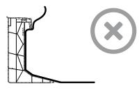
**Incorrect:** roof covering is pulled up over the flange
