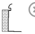
**Incorrect:** roof covering is pulled up over the flange
