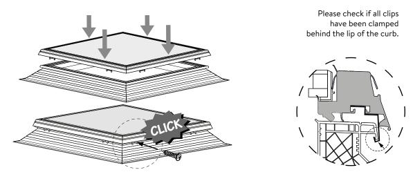
For extra reinforcement, screw the clips through the curb with delivered (one-way) screws.
