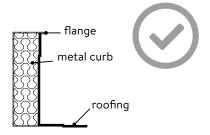
**OK:** roof covering is pulled up to below the flange
