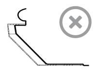
**Incorrect:** roof covering is pulled up over the flange
