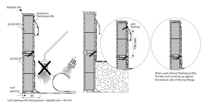
Pull the roofing up to the upper flange. During the hot welding process, make sure to heat the membrane and not the curb.
