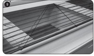
4 Fix the screen on the curb now. Keep in mind that the folded screen does not reach out the border of the curb flange.
