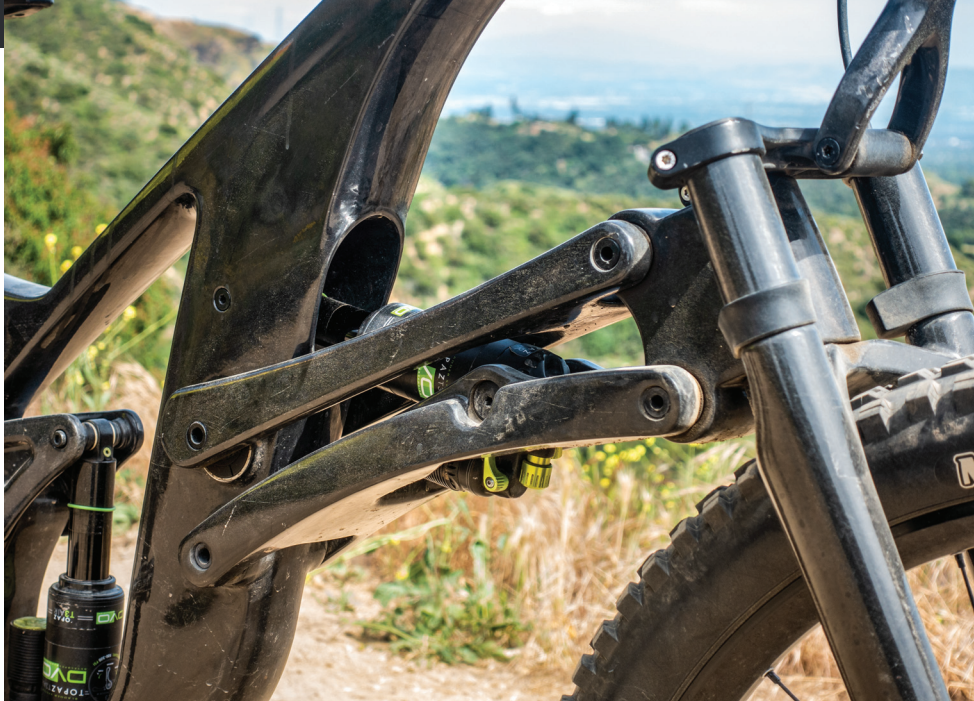
All the bearings in the linkage system are high-precision, sealed-cartridge.
