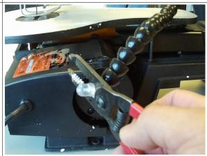
Remove the two Phillips head screws on the snap flex assembly from the upper arm of the saw.
