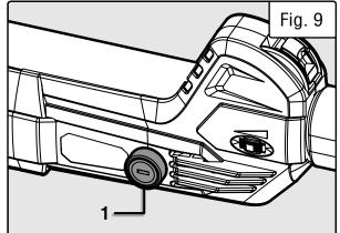
1. Unscrew the brush caps (Fig. 9 - 1) on each side of the motor housing.
