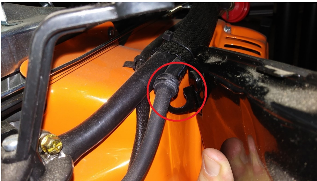
Fig. 7: Disconnect hook on rear of housing from ferrule.
