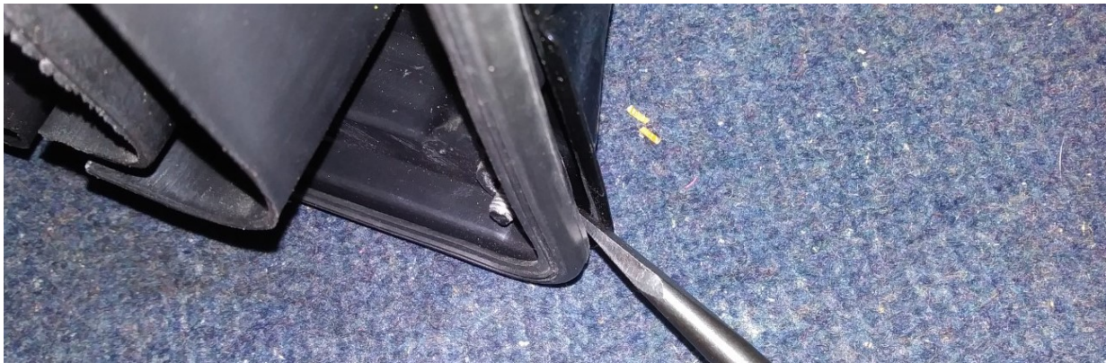
Fig. 3: Use a flat-head screwdriver to gently pry the air filter screen off, if necessary.
