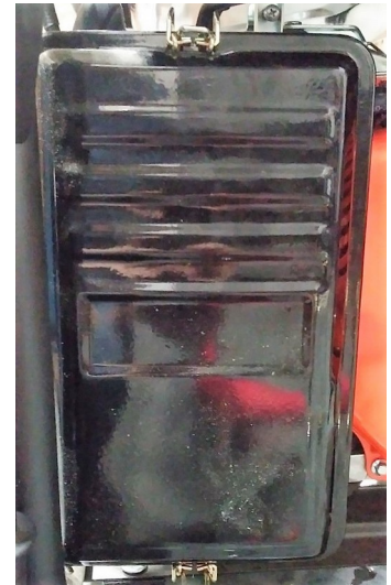
Fig. 12: Air filter cover.
