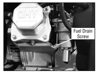
Fig. 14 - Draining the Carburetor
