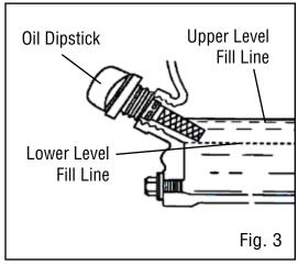
For subsequent operation, the oil level should be checked before each use, or after every 8 hours of operation. The generator is equipped with a low-oil sensor and will NOT start without a sufficient amount of oil.
