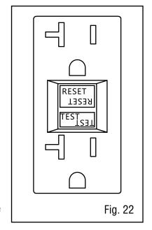
**CAUTION:** If the device does not instantly turn OFF, you may have a faulty GFCI outlet. Call customer service (800) 232-1195 M-F 8-5 CST or email techsupport@wenproducts.com for assistance in replacing the outlet.
