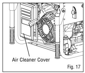
If the air filter element has been damaged, replace it with a new one.
