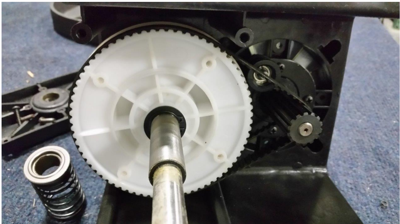
Fig. 9. Pulleys and belts are now exposed.
