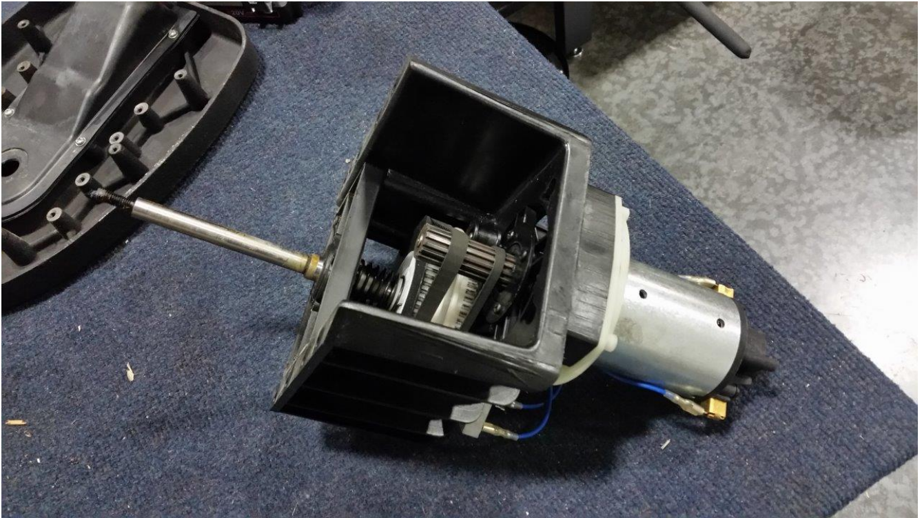
Fig. 6. Remove the motor assembly from the table.
