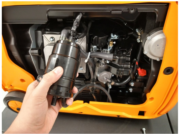
Fig. 3: Position the carbon tank so it hangs near the cylinder head cover.
