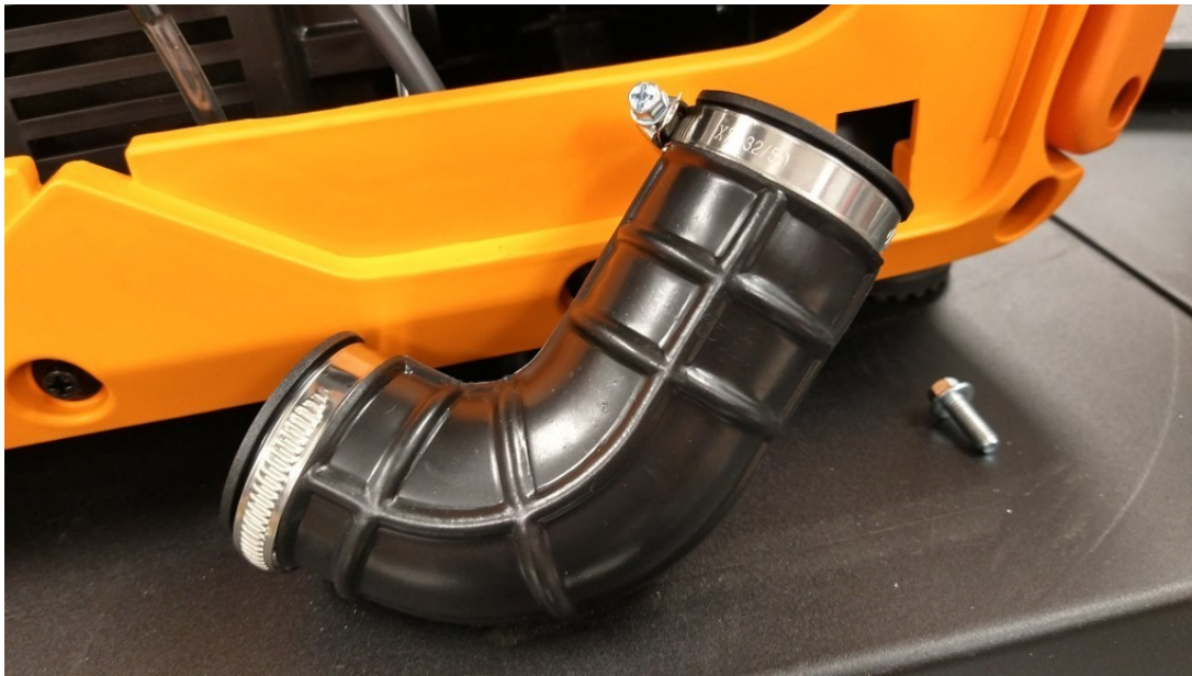
Fig. 5: Air filter duct removed.
