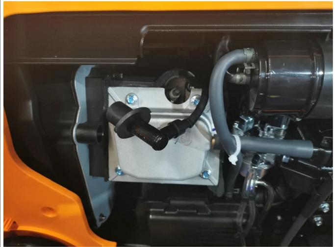
7. Use one hand to hold the ignition coil wiring steady. Twist the spark plug boot off the ignition coil (counterclockwise).
