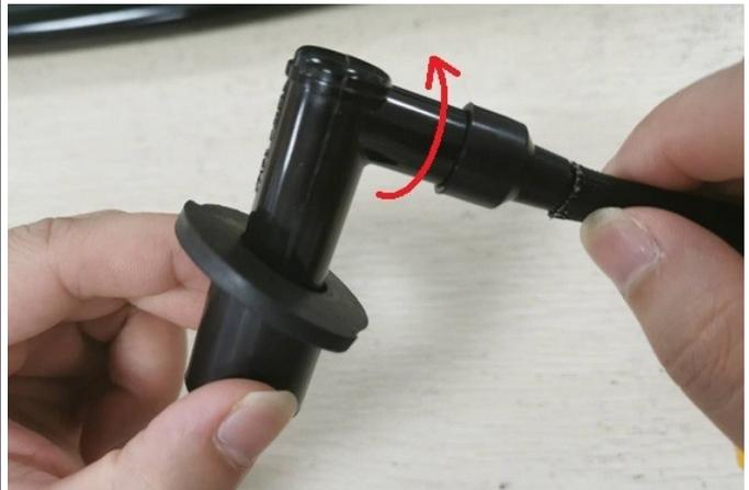
8. Twist the new spark plug boot onto the ignition coil (clockwise) until it is tight. While holding the wiring, tug the spark plug boot sideways to see if it loosens. If so, tighten the boot more. It should not move when tugged.
