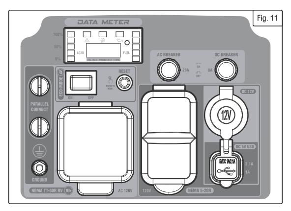
**NOTE**: The NEMA 5-20R receptacles are capable of connecting devices up to 20A only when two generators are parallel connected. When operating a single generator, do not exceed 15.8A (1900 running watts) on this receptacle.
