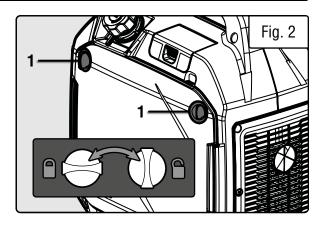
**CAUTION!** For subsequent operation, the oil level should be checked before each use, or after every 8 hours of operation. The generator is equipped with a low-oil sensor and will not start without a sufficient amount of oil. Follow the instructions on the next page to check the oil level.
