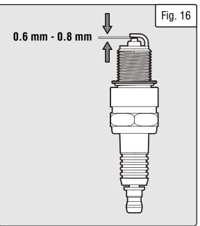
**NOTE:** The recommended tightening of the spark plug is 1/2 to 3/4 of a turn after the spark plug gasket contacts the spark plug hole, or 11.1-14.7 ft-lbs (15 - 20 Nm). Do not over-tighten the spark plug.
