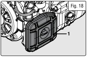
**CAUTION!** Running the engine with a dirty, damaged, or missing air filter element will result in possible danger and cause the engine to wear out prematurely.
