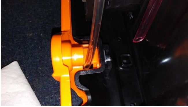
Fig. 17: Drain hose passes through hole.
