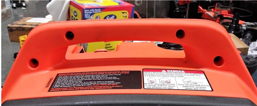
Fig. 12: Remove the 4 Phillips-head screws.
