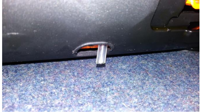
Fig. 18: Drain hose passes through housing
