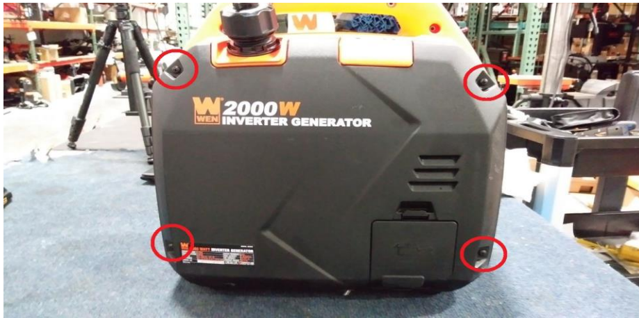
Fig. 1: Remove these screws.
