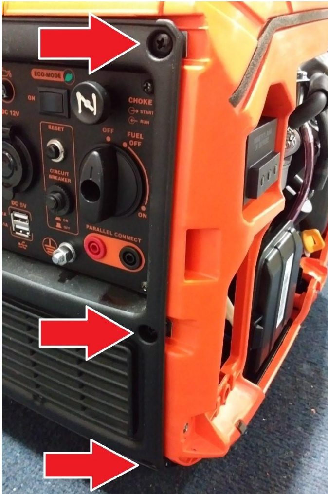
Fig. 9: Control Panel Screws
