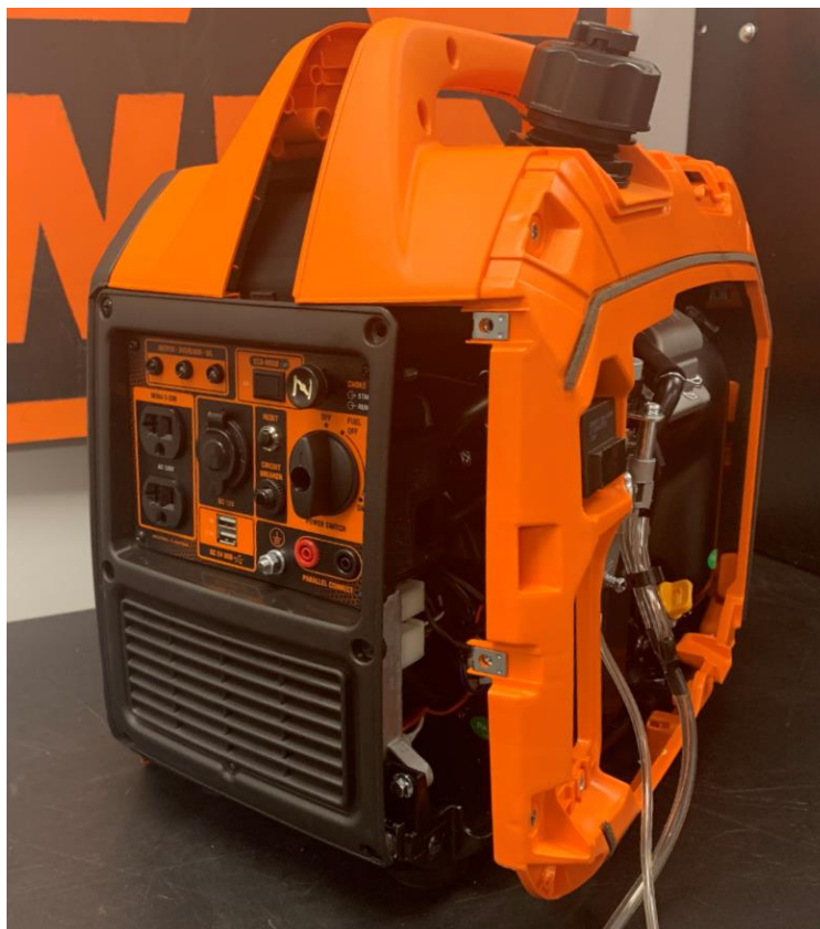
Fig. 13: Loosen the right shell from the generator frame.
