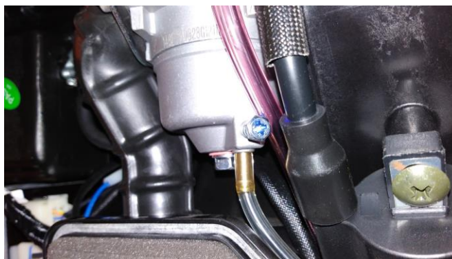
Fig. 3: Carburetor drain screw.
