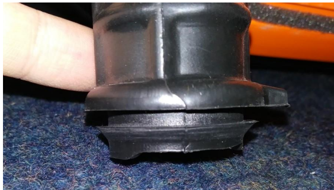
Fig. 16: Barbed fitting on the bottom of the air duct
