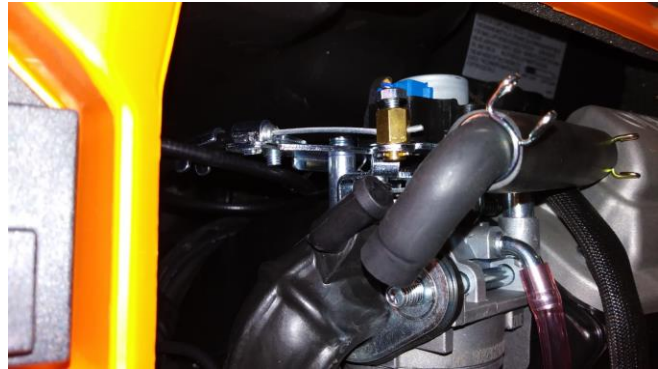
Fig. 5: Breather hose removed from air duct.
