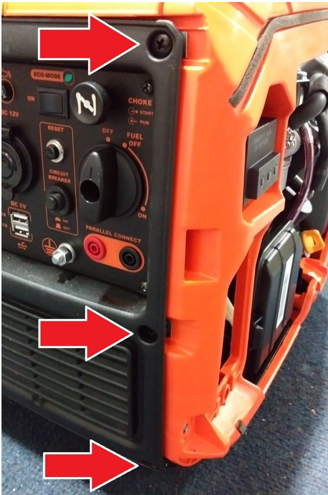
Fig. 2: Remove these screws.
