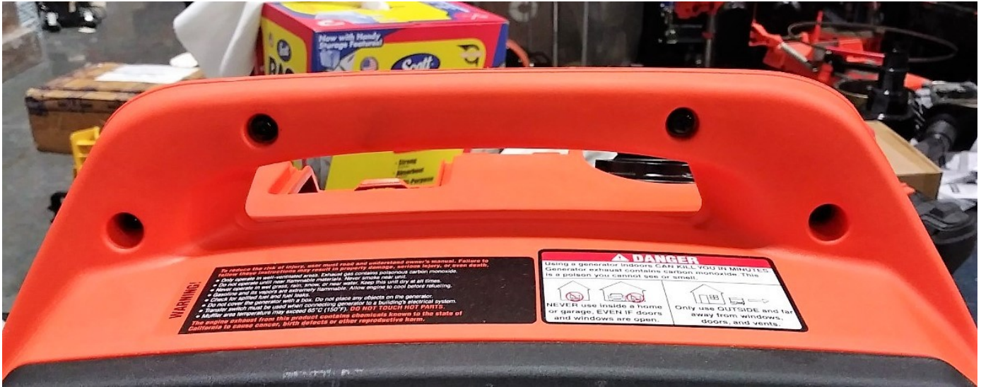
Fig. 5: Remove these 4 Phillips-head screws.
