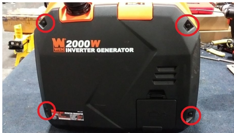
Fig. 1: Remove these four screws.
