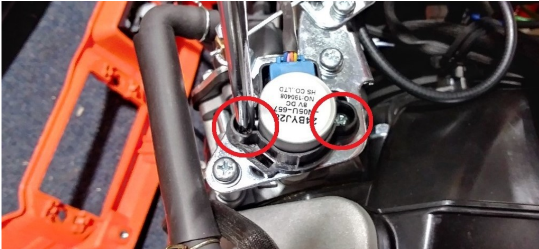
Fig. 7: Remove these two screws.
