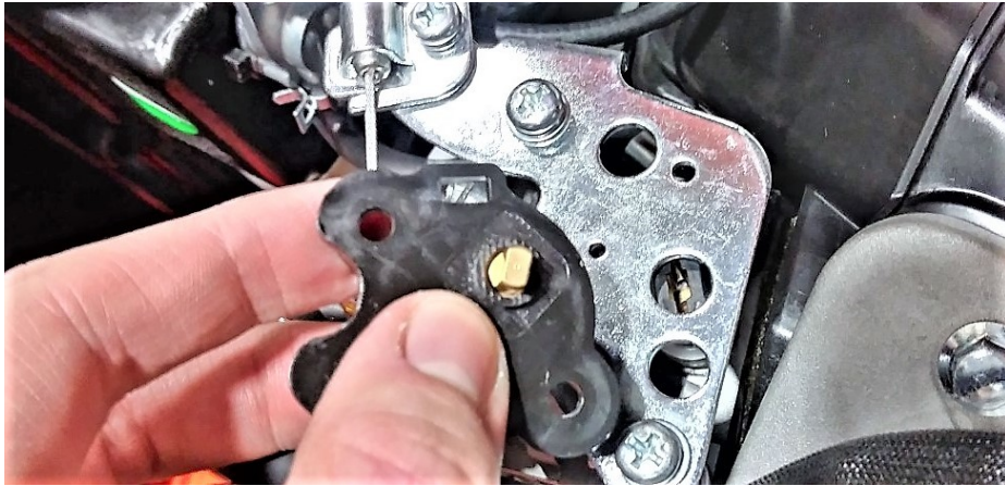
Fig. 21: Stepper motor shaft and throttle must align.
