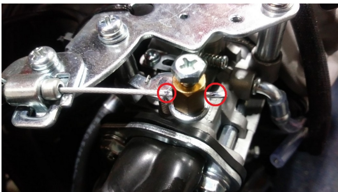
Fig. 10: Mark choke cable on either side of post.
