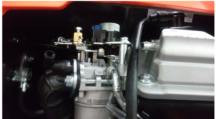
Fig. 9: Breather hose removed.
