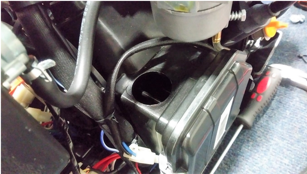
Fig. 20: Hole in air filter housing.
