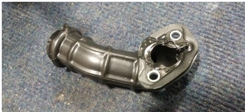
Fig. 15: Air duct between air filter housing and carburetor.
