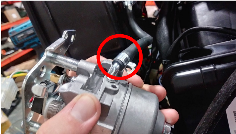
Fig. 16: Remove hose clamp and fuel line.
