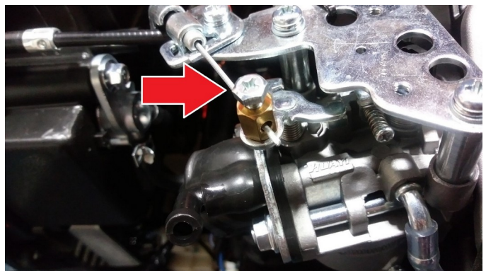
Fig. 11: Loosen choke screw and remove cable.
