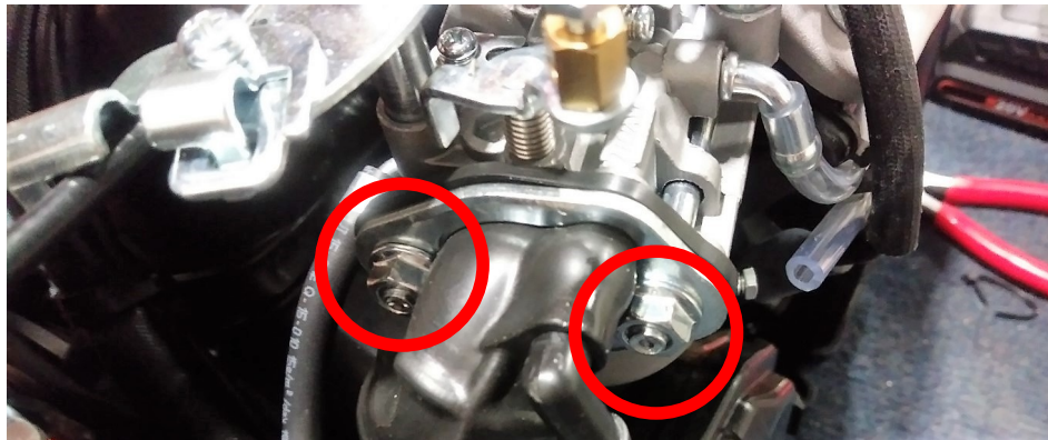
Fig. 14: Remove the two 10mm nuts from the studs.
