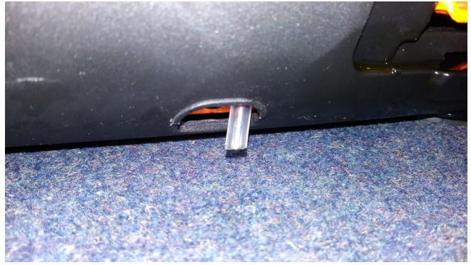
Fig. 11: Drain hose passes through hole.
