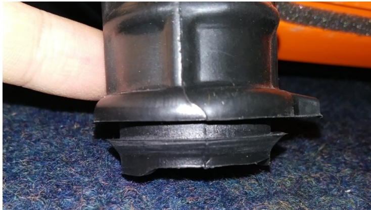
Fig. 9: Barbed fitting on the bottom of the air duct.
