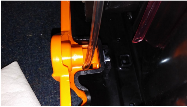
Fig. 10: Drain hose passes through hole.
