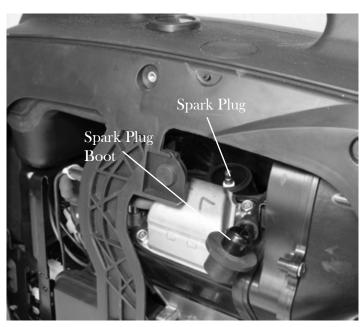
Fig. 11 - Spark Plug Location
