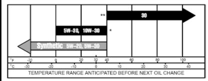
Fig. 1 - Engine Oil Temperature Recommendation
