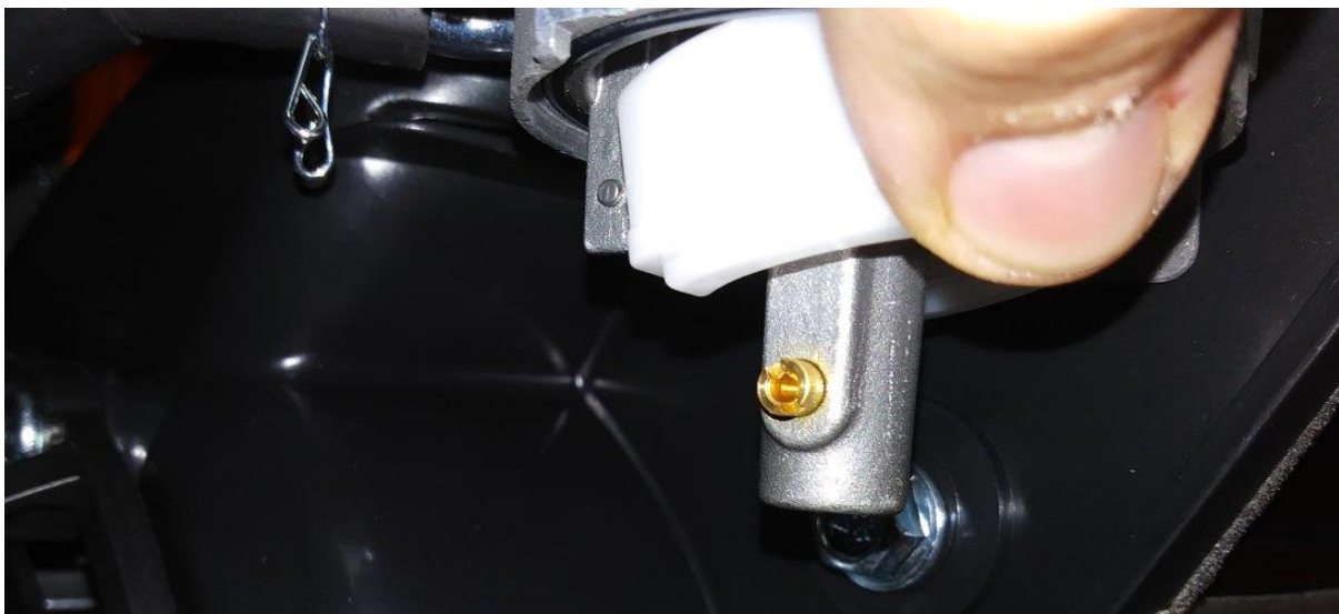
Figure 10: The jet nozzle is shown here, with the float pushed up.
