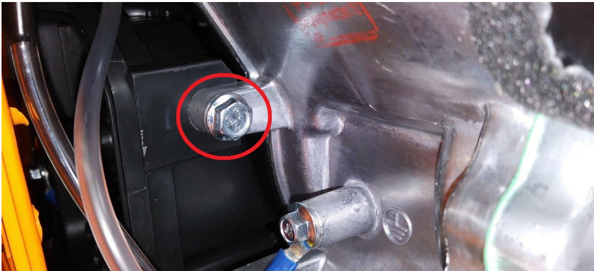
Figure 6: Remove this screw holding the housing to the crankcase.
