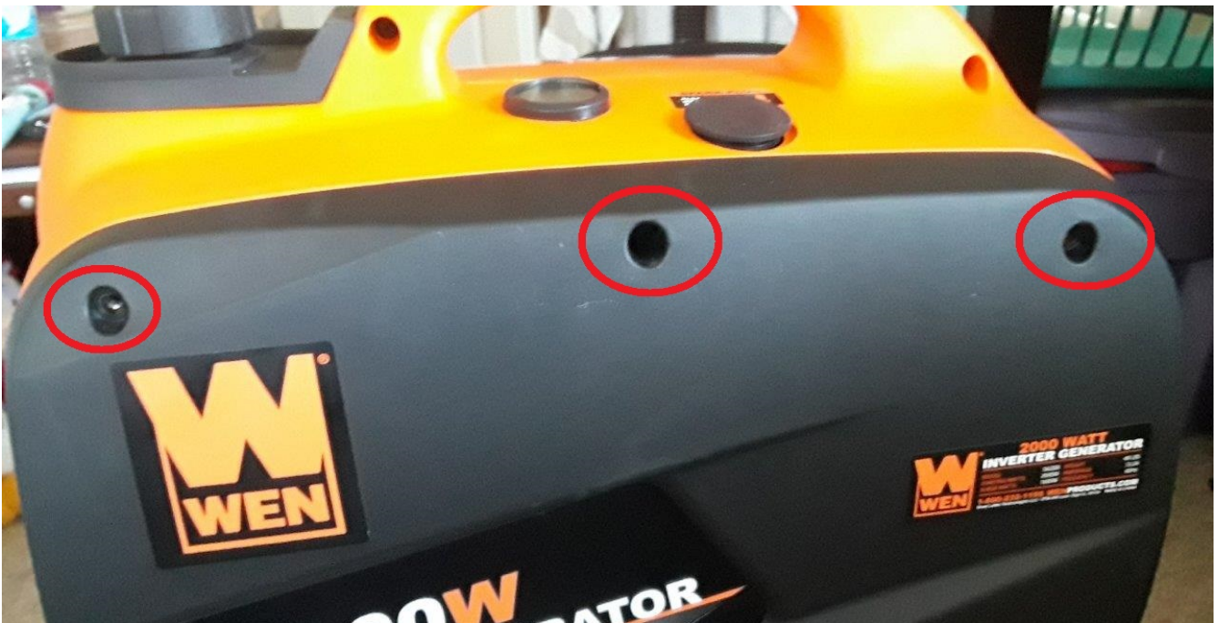
Figure 2: The screws to be removed from the panel.
