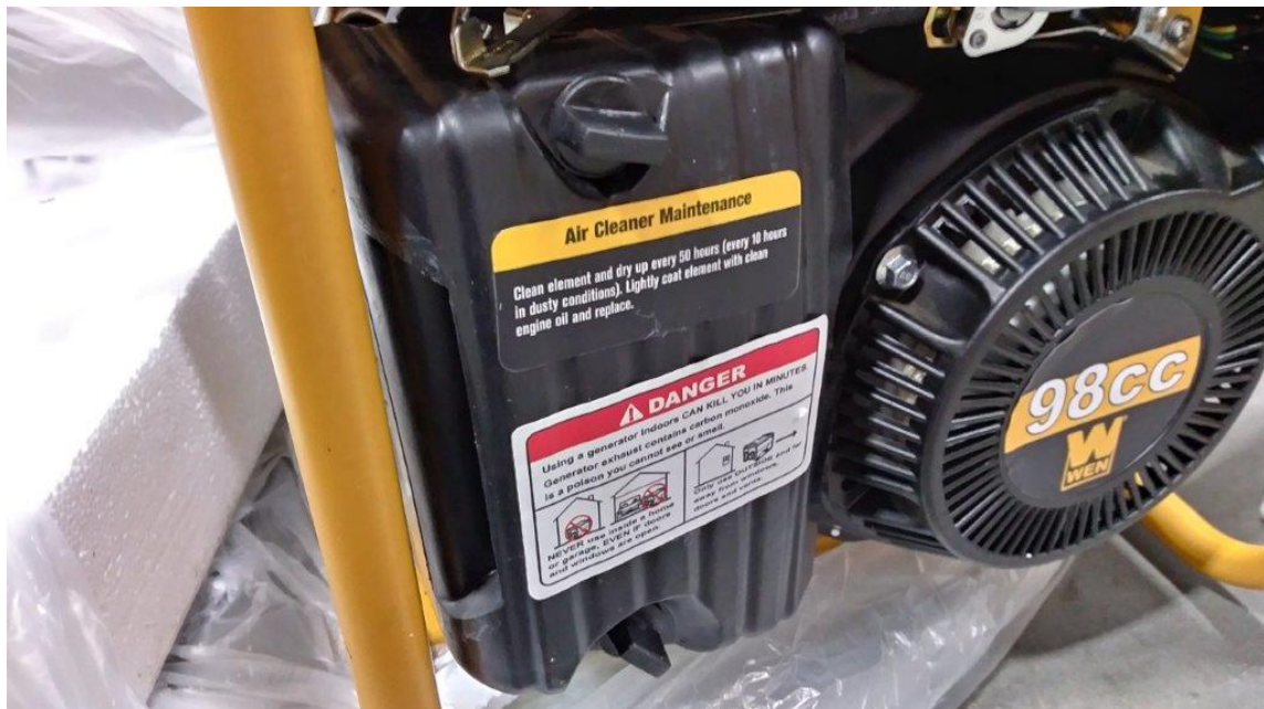
Figure 12: The air filter housing can be removed if you so choose.
