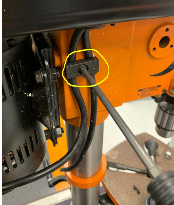
Figure 5. External Motor Cable Clip
