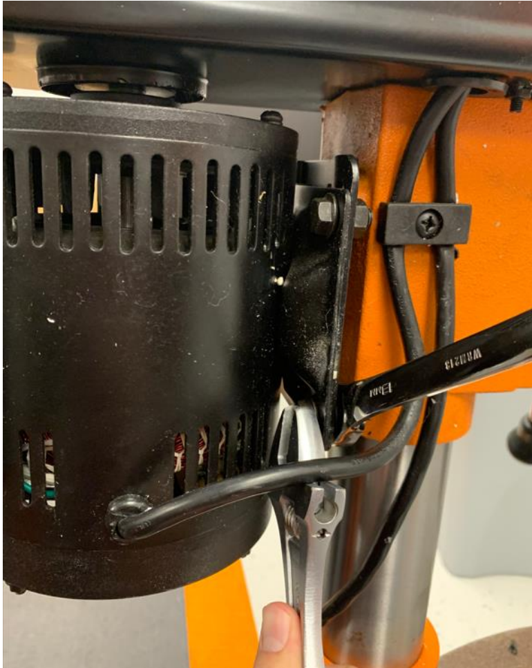
Figure 11. Unbolting the Motor
