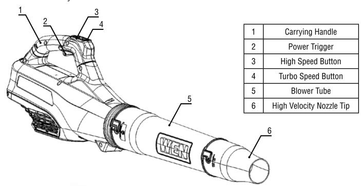
**NOTE:** The high velocity nozzle tip comes packaged inside the blower tube. Remove the high velocity nozzle tip from inside blower tube before operation.
