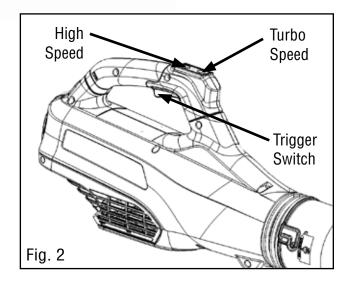
**NOTE:** Turbo speed has been designed to auto-shut off after 35 seconds, reverting the blower back to its low speed.
