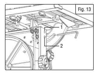
5. Rotate the blade a few times to ensure that the body of the blade does not touch either roller bearing at all while the blade is rotating. Once the bearings have been properly positioned, tighten the screws.
