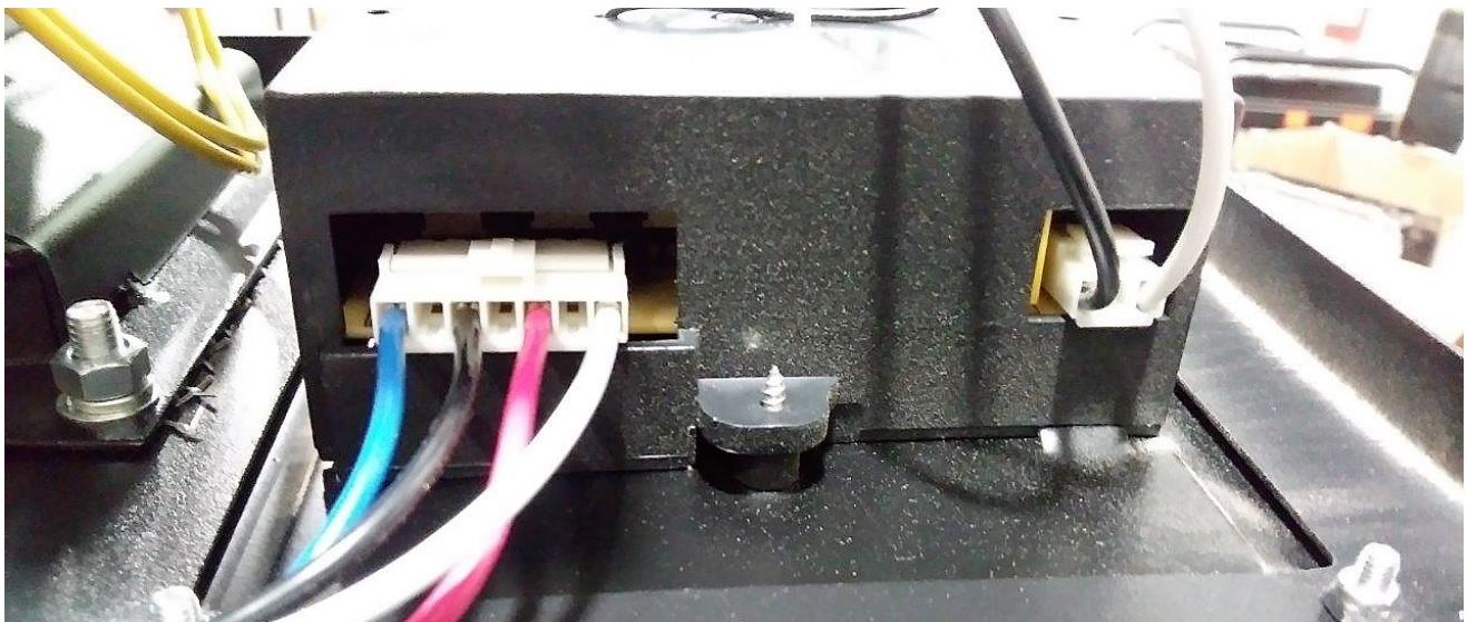
Figure 5: Wired connections to PCB. From left to right: blue, black, red, and white go in slots 1, 3, 5, and 7 (respectively) of the 4-wire connector shown on the left. The black and white wires go in slots 1 and 3 (respectively) of the 2-wire connector shown on the right.
