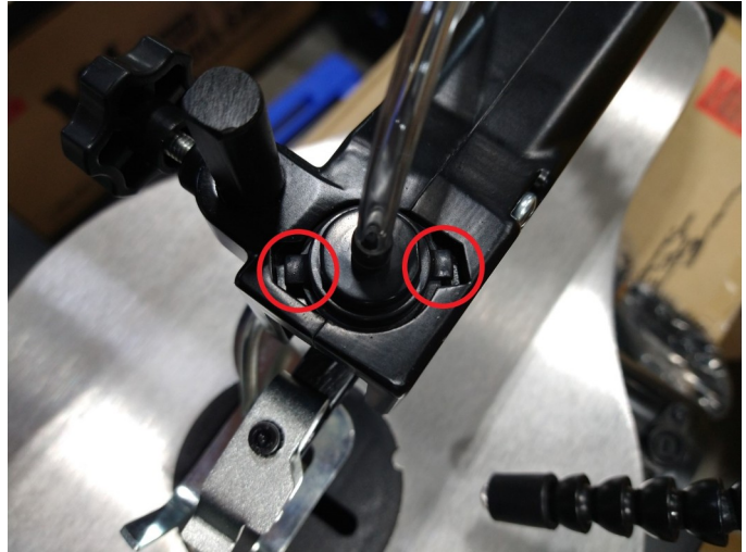
Fig. 3: Cap has been rotated; tabs are aligned with notches.
