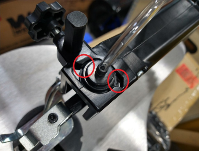
Fig. 2: Tabs are locked in housing.
