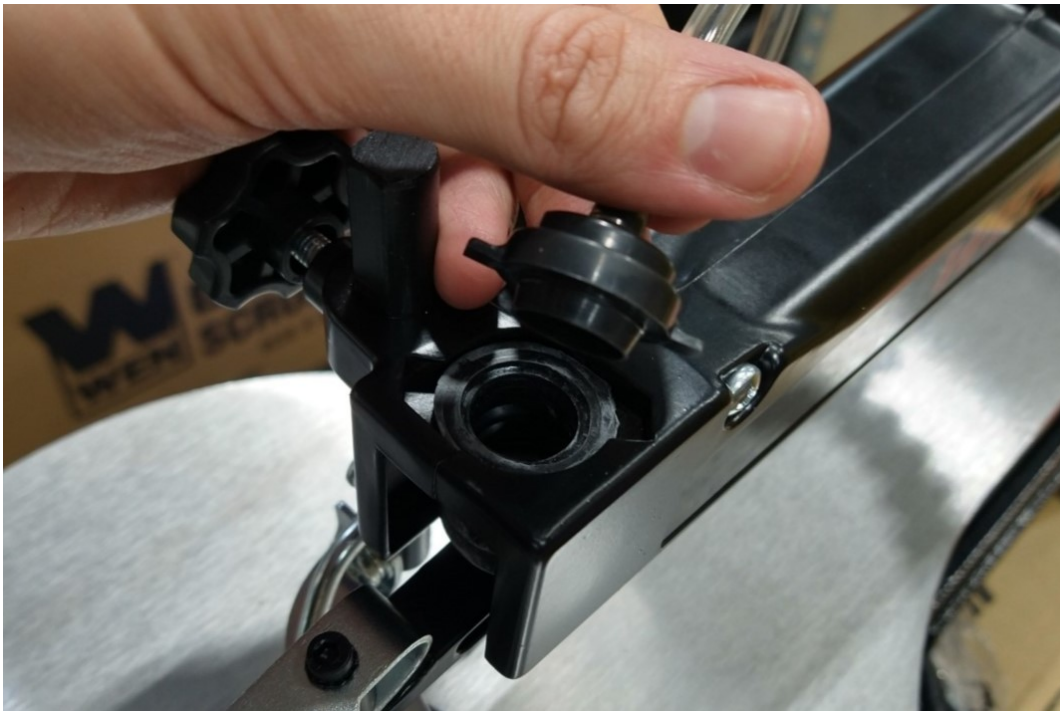
Fig. 4: Bellows cap being lifted off.
