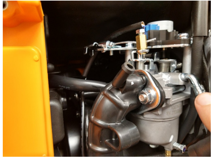
Fig. 5: Breather hose removed.
