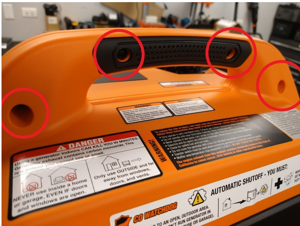
Fig. 12: Remove these 4 Phillips-head screws.
