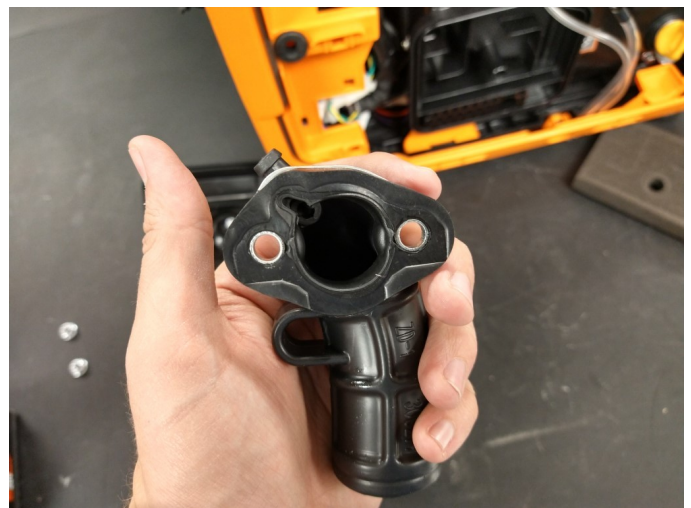
Fig. 9: Remove duct from generator.
