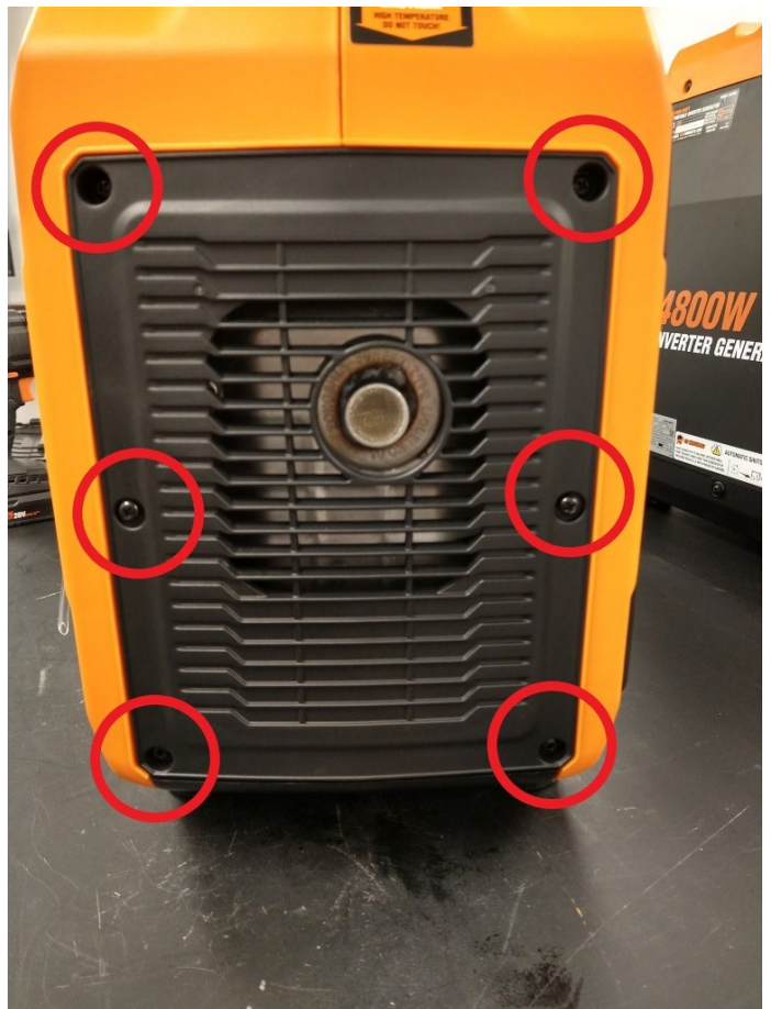
Fig. 15: Remove these 6 screws on the rear panel.
