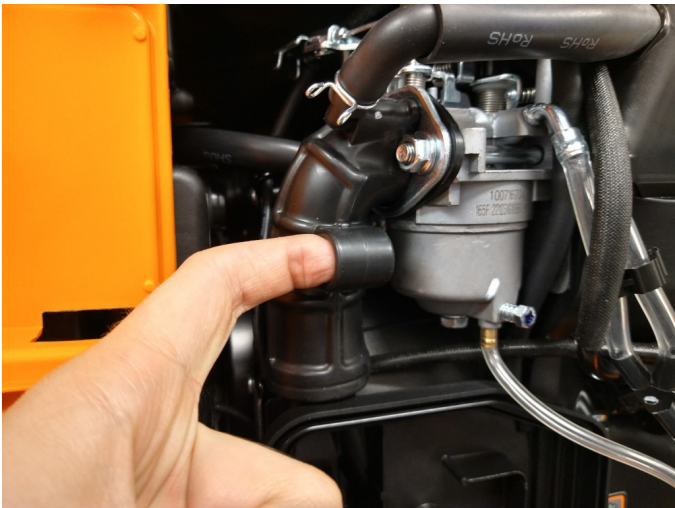
Fig. 6: Tab on air duct to assist removal.
