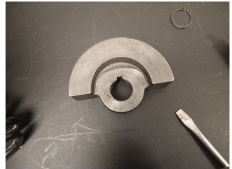
Fig. 17: Eccentric block removed.
