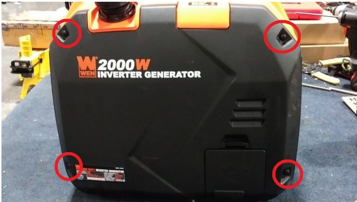
Fig. 1: Remove these four screws (note: oil dipstick and spark plug access panels are still installed as shown here; remove them).
