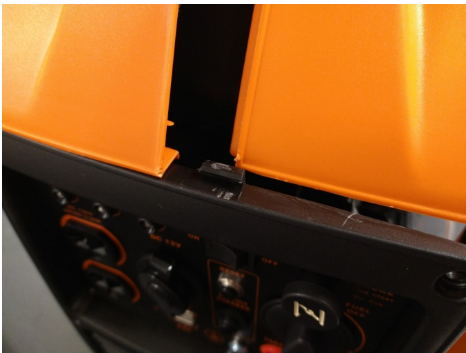
Fig. 17: Control panel tabs.
