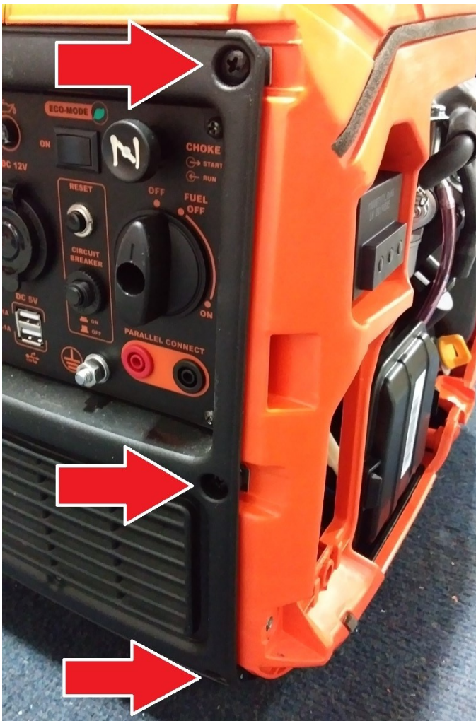
Fig. 3: Remove all 6 control panel screws.
