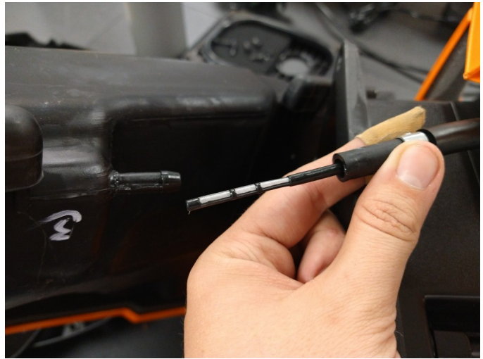
Fig. 10: Line and filter removed from tank.
