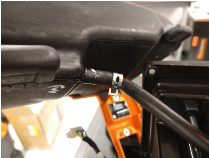
Fig. 9: Hose clamp on the fuel tank.
