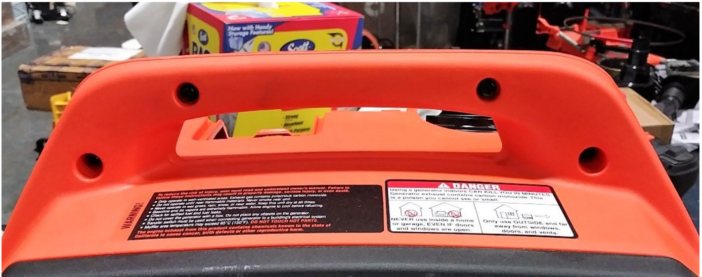
Fig. 6: Remove these 4 Phillips-head screws.
