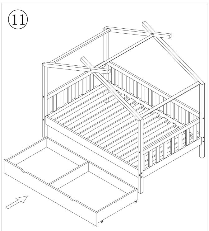
11. Push the drawer under the bed in the direction of the arrow to assemble the whole bed.
