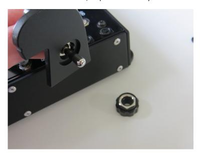
To install the replacement switch you need to detach wires from the old switch. From the factory there will be hot glue covering the ends of the switch wires. Carefully peel this off to expose the metal contacts.
