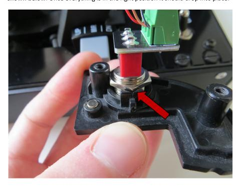
Check the other side of the plate to make sure the switch is in the right position. Only a few threads should come through so the front of the threaded section is roughly in line with the flat surface of the plate.
