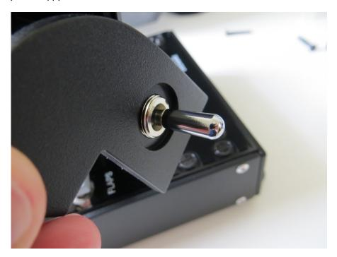
Next use the nut tool again to screw on the outer nut, again if possible try to use the original nut.
