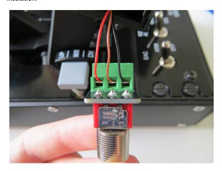
The new switch PCB has the wire colours marked onto it, although you might find it easier to use these two pictures to help you. **Make sure the correct wire goes to the correct terminals.**
