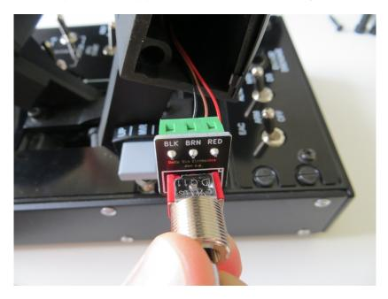
Next take a nut and screw it onto the new sensor. I recommend using a nut that was removed from the throttle if possible, two spare nuts are provided in case the old ones are lost or damaged.
