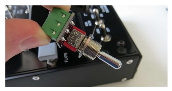
Next install the switch into the throttle side plate, the switch is keyed to the plate so it will only go in one way. The back nut needs to be rotated so it lines up with the slots in the back of the plate, as shown below. Once everything is in the right position it should drop into place.
