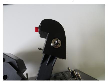
Finally tighten the two screws into the throttle grip to hold everything together.
