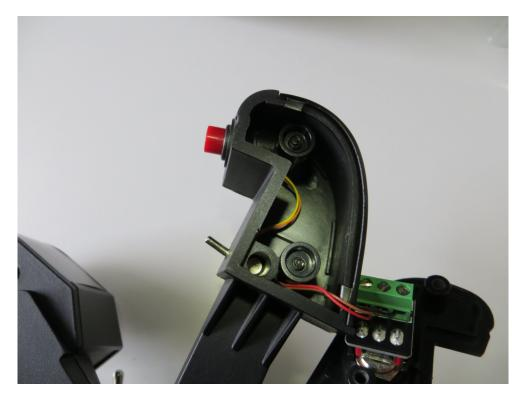
Next put the side plate with the new switch back on, be mindful of where the wire are going inside so you don't crush and damage them when everything it tightened down.
