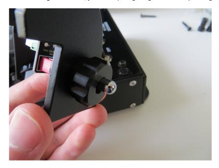
Install the two screws we removed earlier into the two holes on in the throttle.
