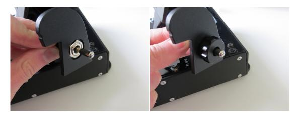
Remove the nuts and switch, keep the nut safe as you will need to reinstall it later.
