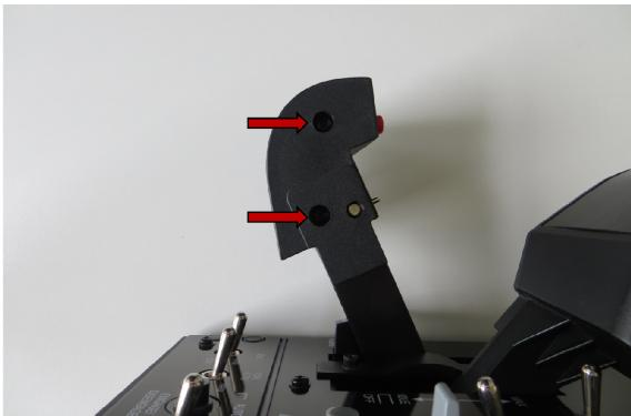
Next unscrew the two screws from the inside of the left hand grip, marked with the arrows.
