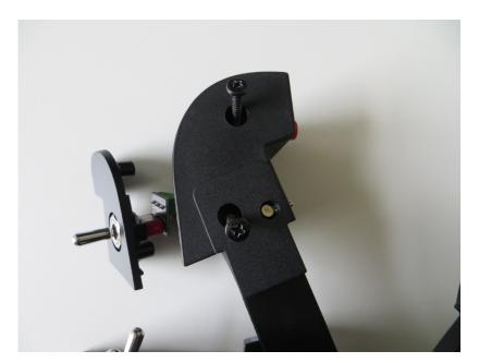
And then install the two plastic pillars over the screws. The larger cup end MUST be at the top, as shown below. You may need to stop the screws falling out of the back with one hand while putting the pillars on with the other. It's much easier to install the screw and pillars now, rather than trying to get everything to line up later.
