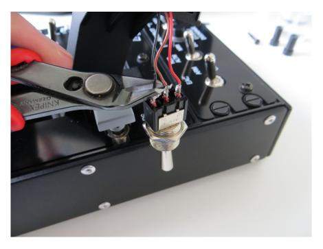
Using a pair or wire cutters or sharp scissors, cut the wires off the old switch. **Do this as close to the switch as you can so you have lots of wire to work with.**
