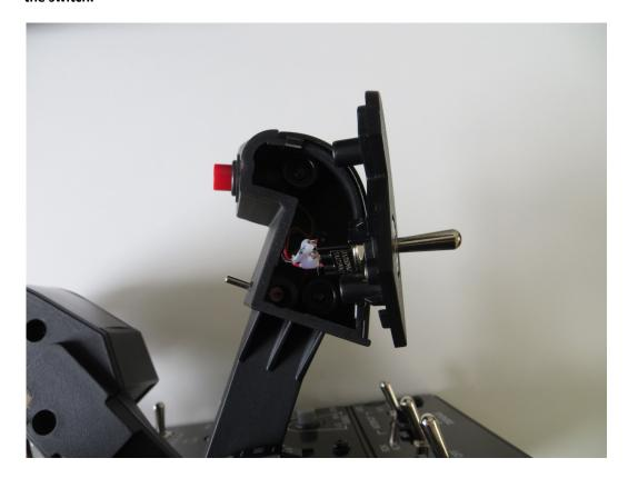
Remove the two screws and plastic pillars from inside the grip, keep these somwhere safe as you need to reinstall them later.
