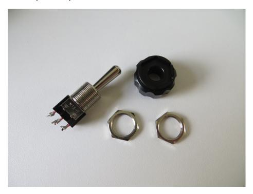
Unscrew the remaining nut from the old switch. You should now have the old switch and two original nuts from the throttle. **Keep the nuts safe as we will reuse these in the next step.**
