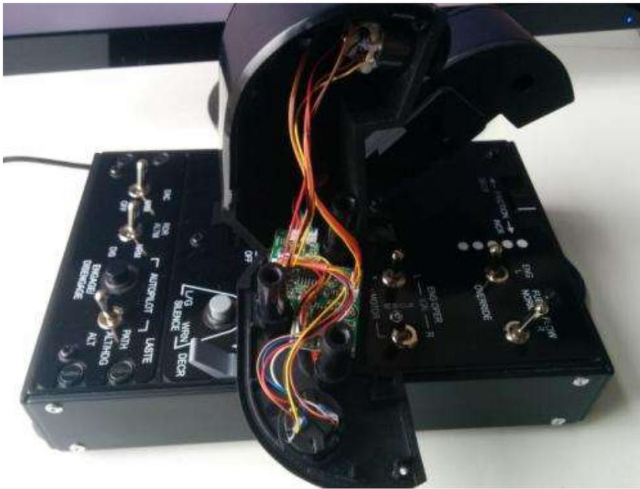
Once the side of the throttle is removed, carefully unplug the old sensor from the throttle PCB.
