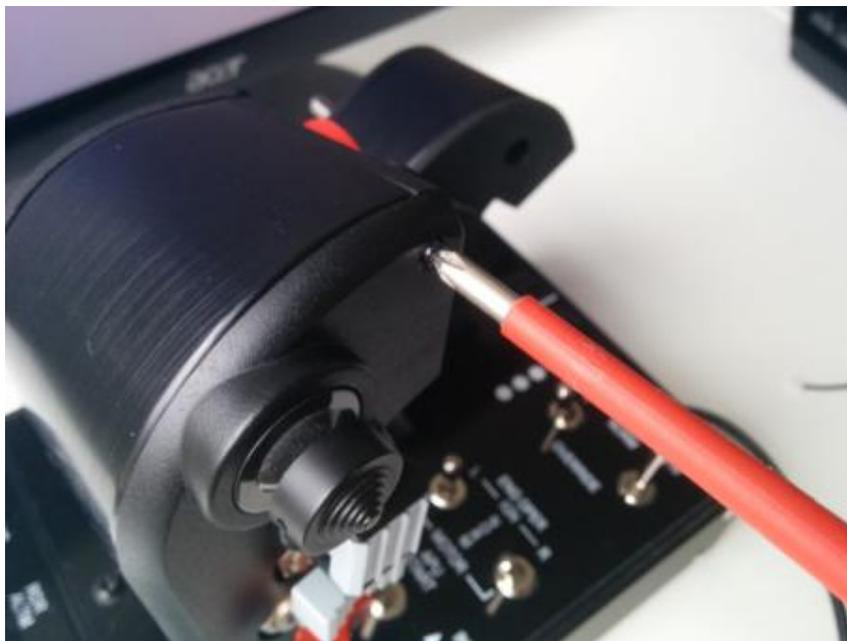
After this is done, I recommend using a bright light to look into the back 3 screw holes to double check all 3 plastic pillars are in place and no wires will be crushed when the screws are installed, if you can see any wires or missing pillars, then you will need to take the throttle apart again to reorganise everything.
