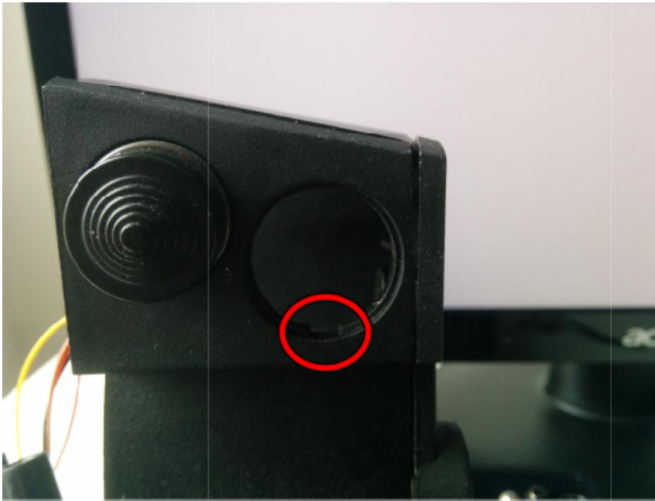
Push the sensor all the way into the throttle until it reaches a positive stop, it should look like the image below, with just a small amount of plastic protruding from the throttle.
