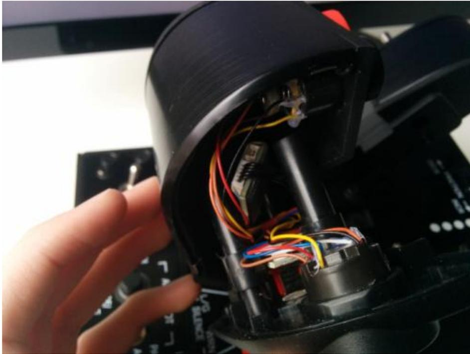
Once the throttle halves are back together, install the small screw into the switch side.
