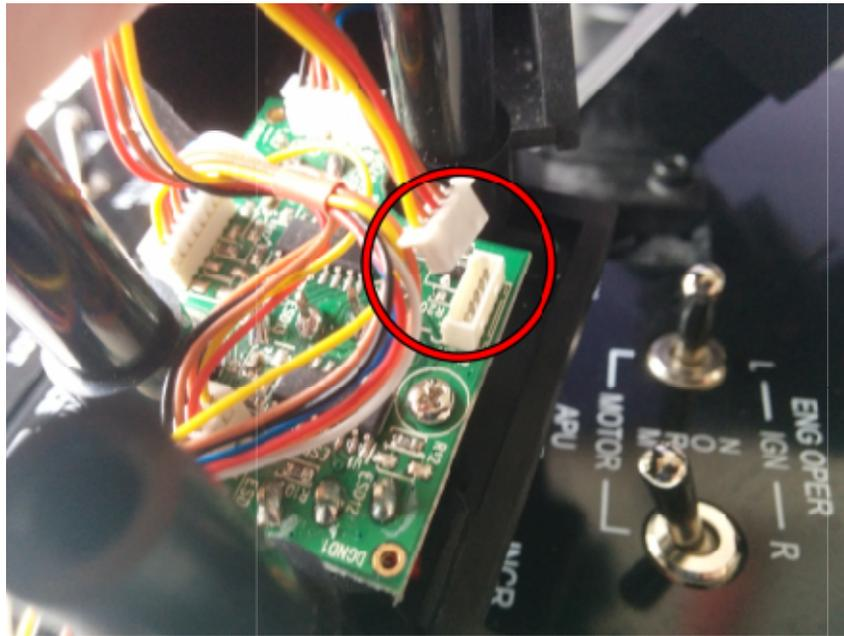
Next remove the old sensor from the throttle housing. To do this you will need to bend the small plastic clips holding the sensor in place. I find pushing them with a finger in the best way to do this. **Do not force the sensor out.** It should come out easily once the clips have been moved out of the way.
