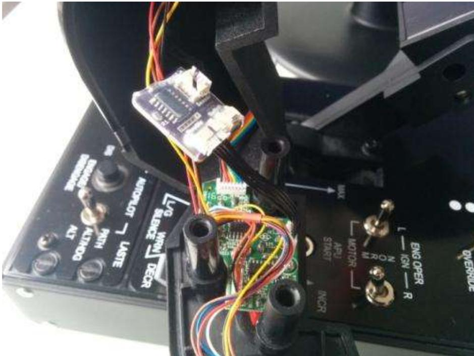
Now you are ready to reassemble the throttle, carefully reorganise the cables back into the throttle. **Take care with the 3 plastic pillars for the screws, they sometimes fall off when putting the throttle back together and are all required to be in place to protect the cables from the screws.**
