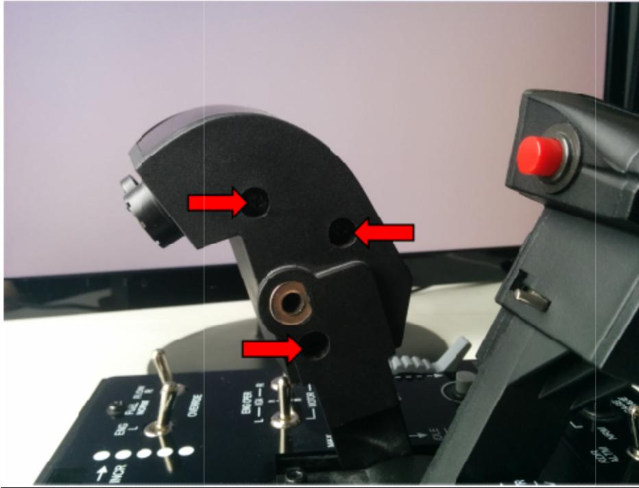
After all 4 screws are removed **carefully** separate the switch side of throttle, take care as wires are connected to both sides and they could become broken this is removed too far.
