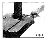
Fig 2. Table Bracket Installation
